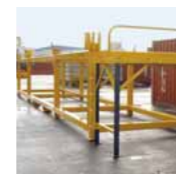
Six-sided inspection rack used as a base so that all six sides of a container can be checked for "hitch hikers".
